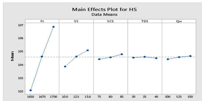
**Fig.5** Main effect plot of Hardness Number Vs. Ft, SS, SCS, TDS and Qw
